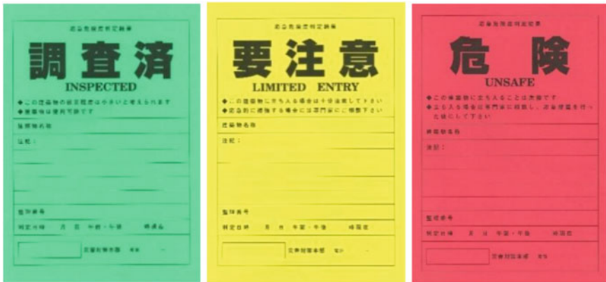
Fig. 2.1 Tags according to the rapid inspection result (Japan building disaster prevention association 2015)
