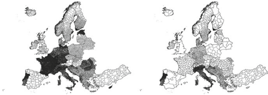
Fig. 7.3 Highest administrative level resolution of the exposure models for residential (left) and commercial (right) buildings
