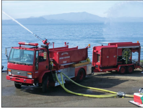
Fig. 13.14 Example of LDH system (Vallejo FD): unit on left is a hose tender with monitor, carrying 5,000 ft. (1,538 m) of 5" (125 mm) hose; unit on right is Hydrosub, a hydraulically driven detachable pump. The pump head can pump 1,500 gpm (6,000 lpm) up to 20 m vertically from a bridge or other point. Here it shown pumping from San Francisco Bay. See Scawthorn (2018) for more details
