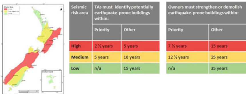
Fig. 1.3 National risk reduction plan in New Zealand (taking effect from 1 July 2017): timeframe for the identification and the remediation (strengthening/retrofit or demolition) of Earthquake Prone Buildings depending on the level of seismicity (low-medium–high seismic areas— PGA < 0.15 g; 0.15 \text{ g} \leq PGA < 0.3 g; PGA \geq 0.30 g)—MBIE 2016
