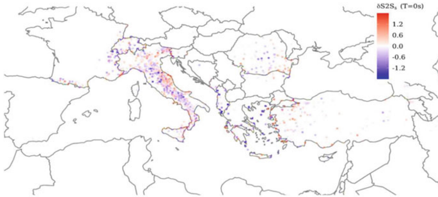
Fig. 11.10 Map illustrating the spatial variability of site-specific ground-motion adjustments. Red markers are sites whose median of the recorded PGA values for past earthquakes was larger than the ergodic median PGA. The opposite holds for the median PGA at the blue marker locations. The adjustments, expressed in terms of the \delta S2S_s quantity mapped here, were estimated from the Engineering Strong Motion dataset by Kotha et al. (2020)
