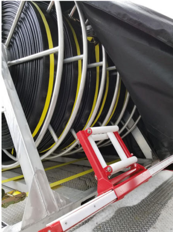
Fig. 13.15 Vancouver (B.C.) Fire and Rescue new LDH reel system—each trailer-mounted motorized reel carries 6000 ft. of 6" hose. Photo Scawthorn (2019)
