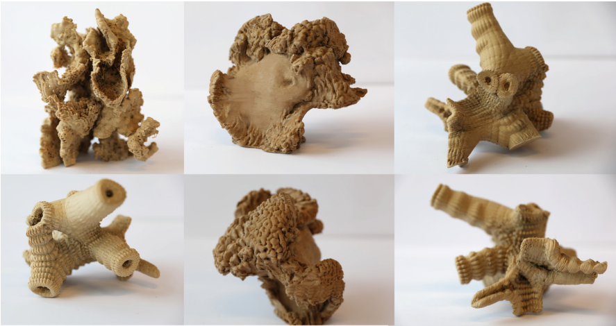
Fig. 5. 3D printed scaffolds from wood based biodegradable plastic infused with corn starch and natural fibers.
