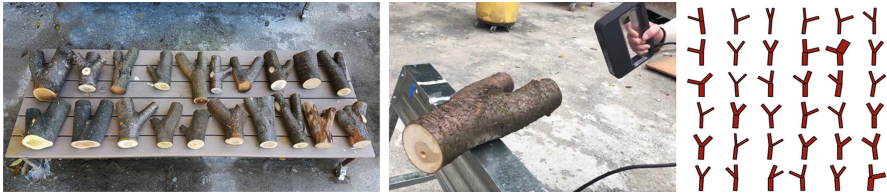
Fig. 7. Sourced crotches are 3D-scanned to establish the material library
