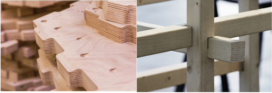
Fig. 1. Example of a finger joint with additional fasteners (left) and integral joints (right). Source: ICD, University of Stuttgart (left).
