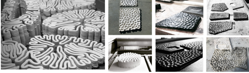
Fig. 6. Material formation of the bio-tile
