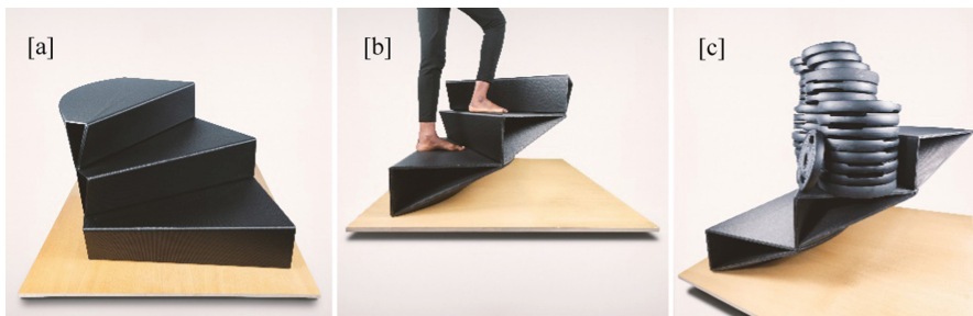
Fig. 6. Configuration 2, Photographs of three modules prototype. (a) Front, (b) Side, (c) 2452 N payload test.
