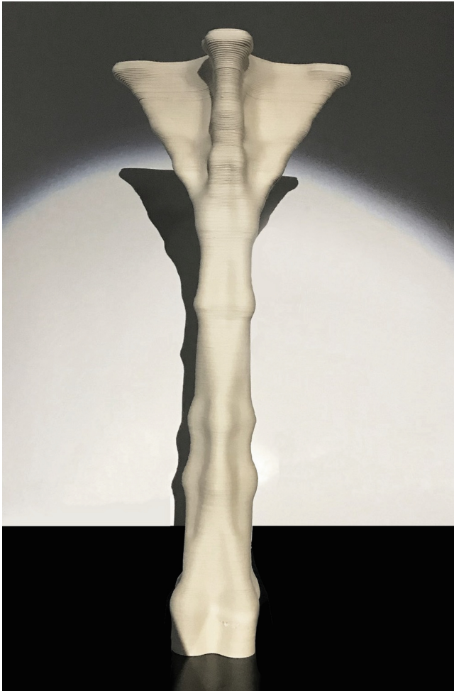
Fig. 30. Printing parameters. Prototype height: 1 m. Max decline angle: 40 ° Prototype Weight: 3.25 kg Total Routine Length: 202 m Nozzle Diameter: 4 mm Material Amount: 8080 cm Printing Time: 6 h 25 min
