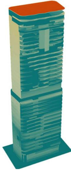
**Fig. 7.** Grasshopper/Rhino 3d definition showing environmental analysis. Relative humidity Each colour represents a different microclimate. The colours result from the cross-reference between the environmental analysis and the microclimate parameters. (3D image by author)
