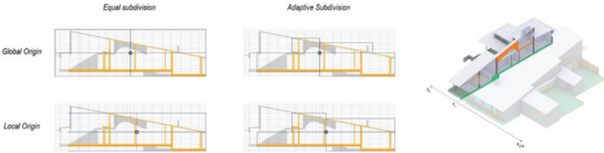
Fig. 2. Global versus local subdivision. Four distinct strategies for slice-subdivision. Top left: Equal slice-subdivision with global origin. Top right: Adaptive slice-subdivision with global origin. Bottom left: Equal slice-subdivision with Local Origin. Bottom-right: Adaptive slice-subdivision with local origin.
