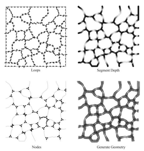
**Fig. 9.** Analysis of a generated network. New geometries can be generated along the path, and based on their relationship to network nodes. We can notice that three-connection nodes are most common in generated patterns (bottom left), which are also approximately averagely divided.
