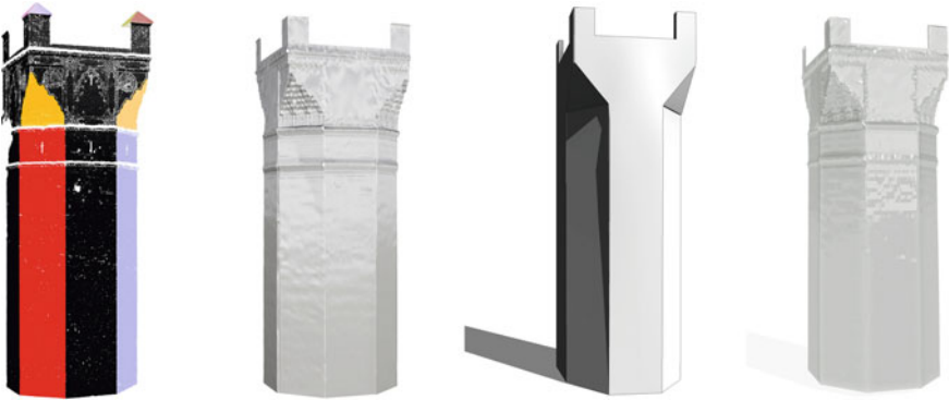
Fig. 7. Chellah tower. From left to right: Segmented point cloud, mesh reconstruction, BIM model LOD 100, BIM model LOD 400.
