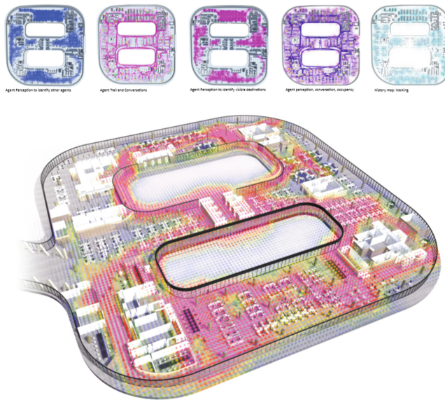
Fig. 8. ZHA ABPS's example data analysis on Infinitus headquarter project, which shows the different social interaction patterns and analysis, such as agent perception, conversation, occupancy, history map, etc. (credit: Tyson Hosmer (team leader), Soungmin Yu, Sobitha Ravichandran, and Ziming He)
