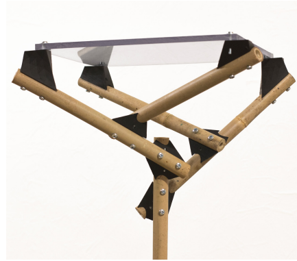
Fig. 25. Finished structure. Successfully interfacing with plate through adapting the geometries of pole-to-plate connectors
