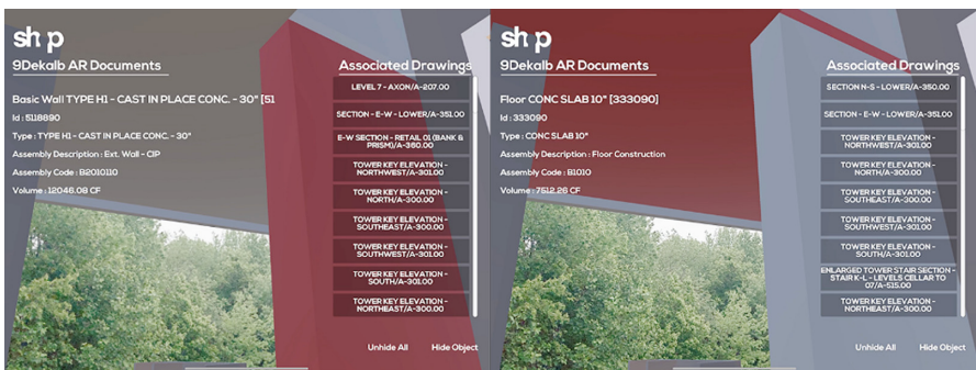
Fig. 2. A screenshot showing the information and associated views of a selected model element
