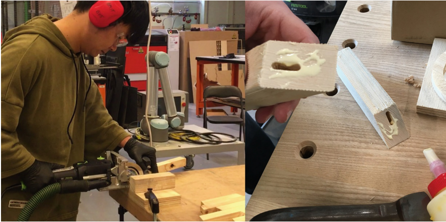
Fig. 5. A standardized timber domino system was used to fix the parts of the aggregation together cutting process were used to stitch and brace these chunks together to enhance structural stability of the aggregation (Fig. 6).
