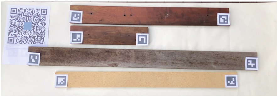
Fig. 7. Individual Aruco markers can be placed on top of each timber offcut and aligned to a QR Origin code
