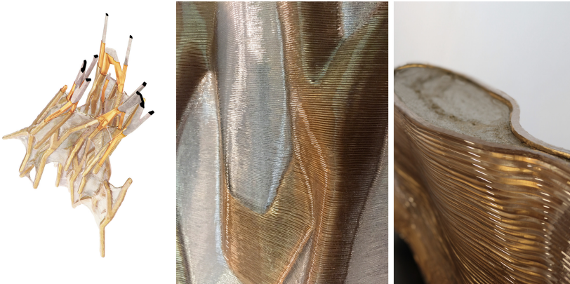
Fig. 4. Concrete infused sacrificial formwork, NGV Pavilion, 2016, Studio Roland Snooks
