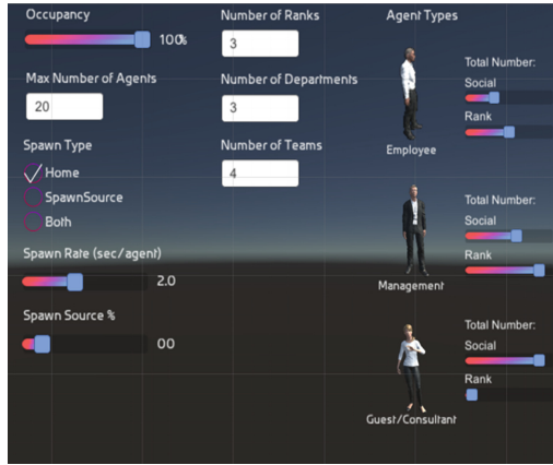
Fig. 7. ZHA ABPS's example interface of agent types, in the working scenario, the agents can be classified into different working teams, and agents can be differentiated as team leaders who will have more meetings, and team members who will work at the desk more. And each agent contains a set of different needs parameters, like thirst, hunger, concentration, motivation to work, etc. (credit: Tyson Hosmer (team leader), Soungmin Yu, Sobitha Ravichandran, and Ziming He)
