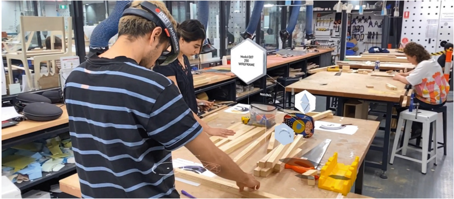
Fig. 4. A holographic interface was used to update aggregation parts for a dynamic nesting in the offcut scraps
