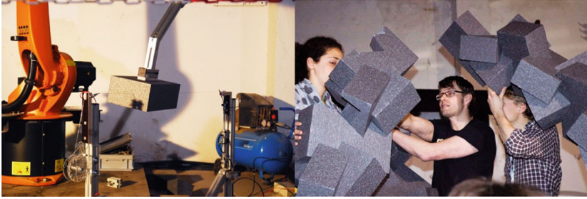
Fig. 3. Robot arm hot-wire cutting process (left) and result (right).
