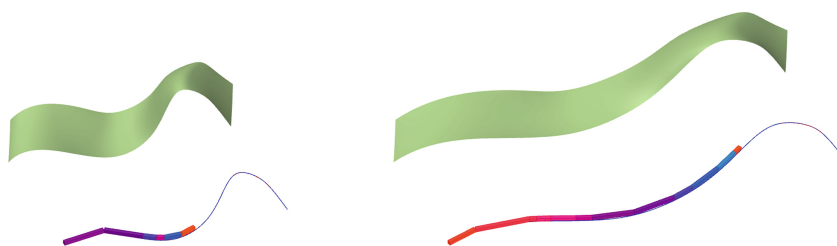
Fig. 11. Adjusting the digital model to increase efficient use of timber lengths
