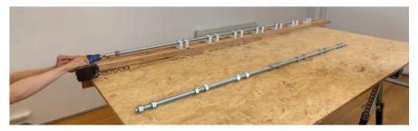
Fig. 13. After all the hex nut locators were properly placed, a threaded rod is screwed through jig
