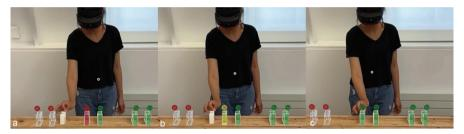
**Fig. 12.** *Object calibration* is employed to ensure the hex nut locators are adjusted to match the digital model. As the physical hex nut locator moves closer to its digital position, the notation would transform from red to yellow to green.
