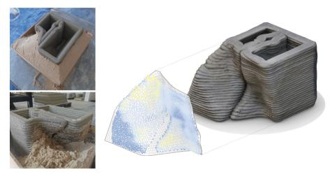
**Fig. 7.** Section print test of one of the prototypes, using sand as support material (left) and analysis of the photogrammetry model obtained with the target geometry (right).
