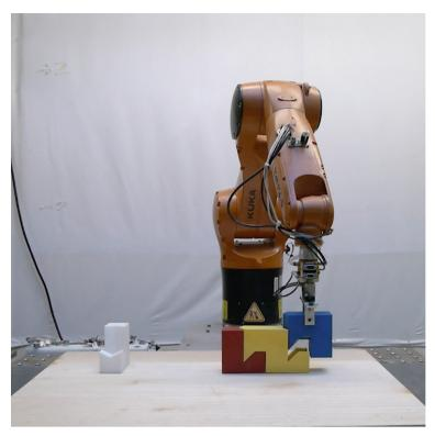
Fig. 2. The robotic construction of 3D-Printed interlocking units. Where unit shape C' is added to unit shape B'
