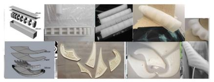
**Fig. 4.** Programable Soft Materials: TPU and silicone and the process of their computed structures supported by Rhino and CAD. The Fig. 3 shows the process of TPU computed structures which was supported by Tongji University College of Architecture and Urban Planning and developed in DigitalFUTURES Shanghai 2018 Workshop
