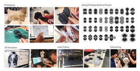
**Fig. 3.** Programable Soft Materials: TPU and silicone and the process of their computed structures supported by Rhino and CAD. The Fig. 3 shows the process of TPU computed structures which was supported by Tongji University College of Architecture and Urban Planning and developed in DigitalFUTURES Shanghai 2018 Workshop
