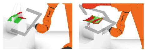
Fig. 7. Simulation of hot wire cutting process in grasshopper
