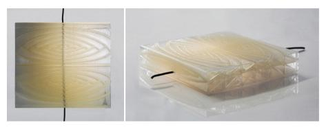
Fig. 11. FDM printed 1:8 scale module.
