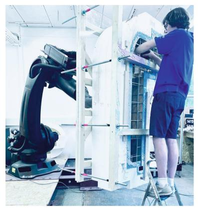
Fig. 8. Robotic sequential casting (RotoForm) process pouring the calculated amount of mortar inside the dynamic formwork.
