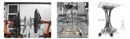
**Fig. 2. a** Two robots share a workpiece (Prado et al. 2014) **b** 6-axis robot exchanges fiber with 2-axis gantry (Duque Estrada et al. 2020), **c** Two mobile robots manipulate fiber bobbins simultaneously (Tucker et al. 2022)
