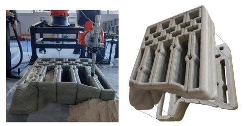
**Fig. 9.** Printing process of a full-scale prototype (left) and post-tensioning aggregation scheme of two printed sections (right).
