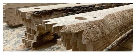
Fig. 8. Robotically Kerfed logs with finger joints and threaded rod holes
