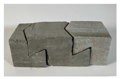
Fig. 3. Design of interlocking concrete assembly using custom units A'B'C where units form components of a wall structure
