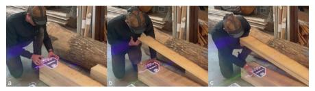
Fig. 7. *Object identification* is utilized to identify physical components and display intuitive step-by-step assembly instructions.
