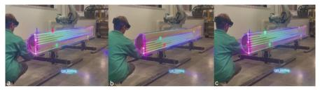
Fig. 5. *Object localization* is used to determine the placement of the toolpath for robotic fabrication.
