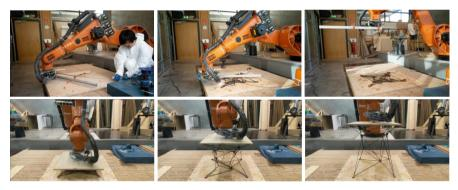
Fig. 17. a Semi-robotic winding of early prototype b Deployment of prototype structure
