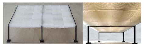
Fig. 10. FDM printed 1:25 scale modules assembled with iron wires.
