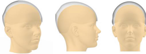
Fig. 2. Custom-fit helmet shell
