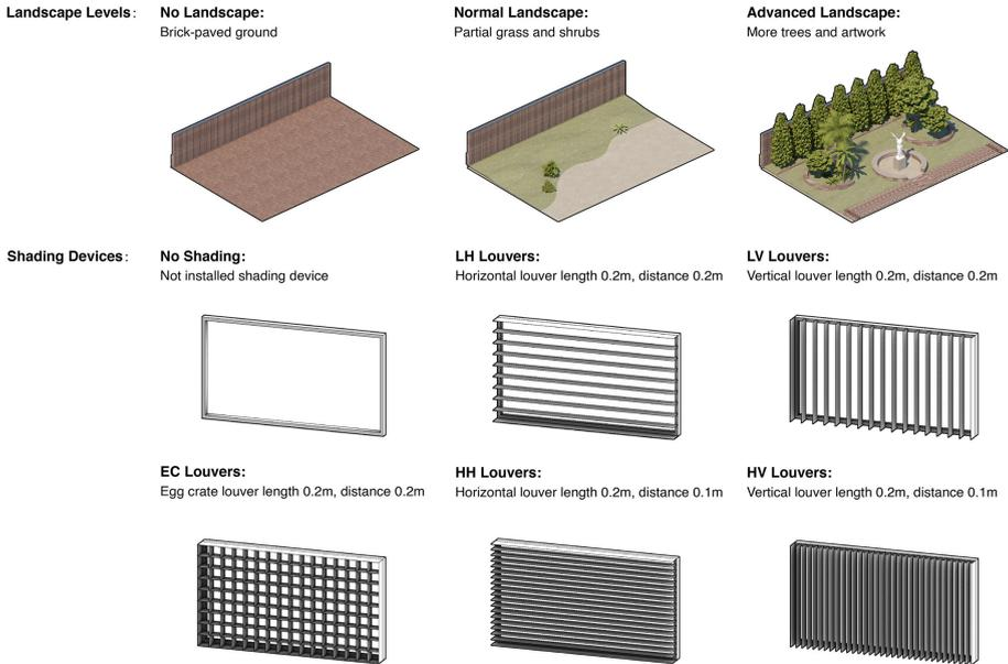
**Fig. 3.** Three different landscape levels and six different shading devices for window view analysis.
