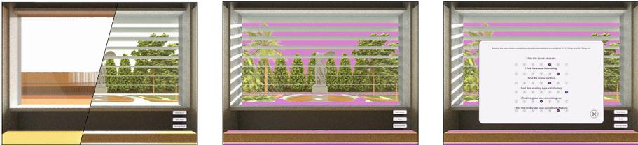
**Fig. 5.** The three main functions of the VR window view evaluation tool: scene-switching function (left), glare observation function (center), and evaluation function (right).
