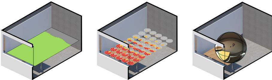
**Fig. 4.** Example of sensor points with views used for sDA simulations (left), sDG simulations (center), and window view rendering (right).
