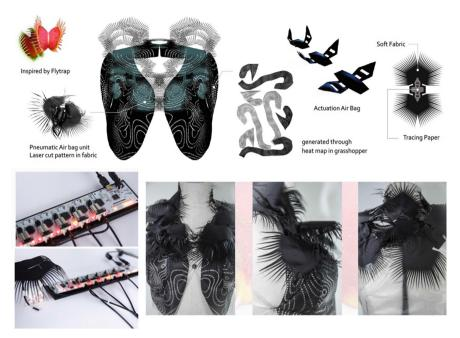
Fig. 7. Various prototypes of pneumatic air-bags' structures inspired by muscles and flytrap
