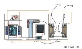
**Fig. 6.** An example of pocket-sized pneumatic system with one portable air pump, one pair of two-sets miniature electromagnetic valves that can control two sets of airbags, and an Arduino toolkit which can connect sensors easily
