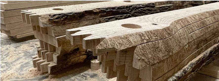
**Fig. 8.** Robotically Kerfed logs with finger joints and threaded rod holes
