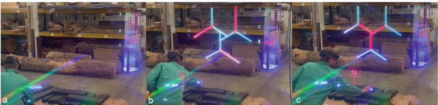
**Fig. 10.** *Object identification* is utilized to identify physical components and display part to whole assembly instructions.
