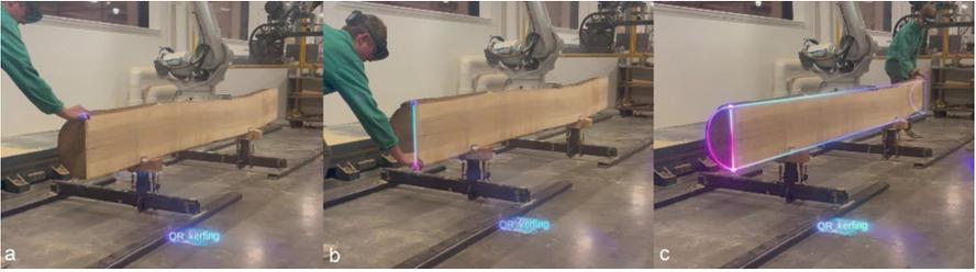
**Fig. 4.** *Object localization* is used to determine the work object placement for robotic fabrication.
