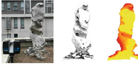
Fig. 3. 3D scan of a natural Taihu rock and the analysis of its geometric characteristics.
