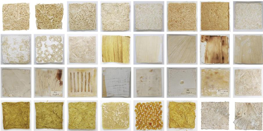
**Fig. 3.** Different combination of maize kernels, fibres and binders
