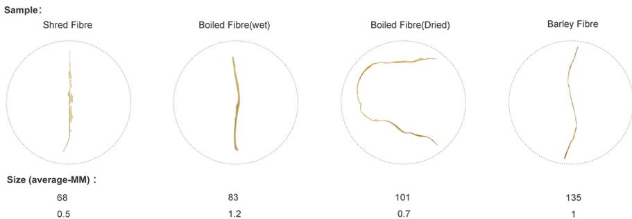
**Fig. 2.** Comparison of fiber properties by different techniques
