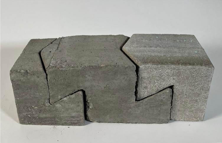
**Fig. 3.** Design of interlocking concrete assembly using custom units *A' B' C* where units form components of a wall structure
