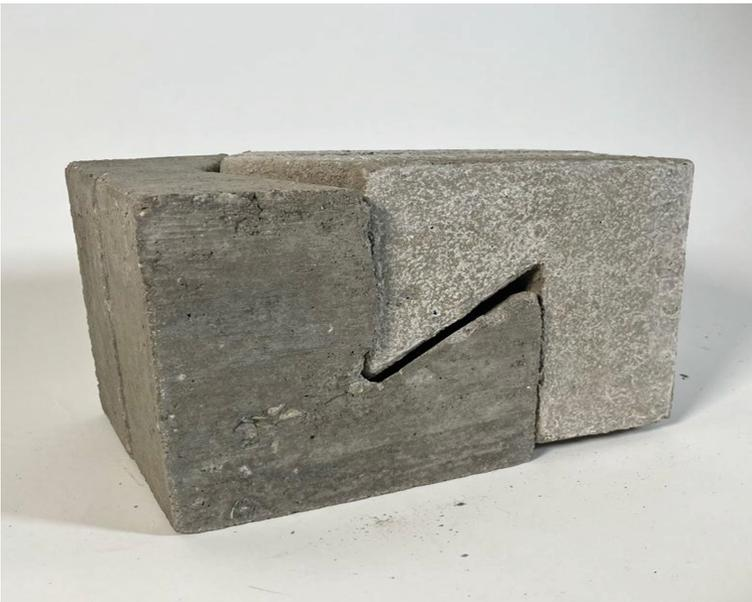
**Fig. 4.** Design of interlocking concrete assembly using custom units *A' B' C* where units form components of a wall structure
