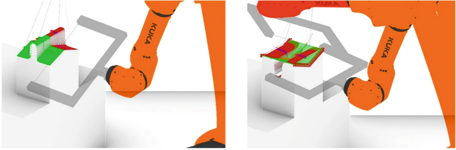
Fig. 7. Simulation of hot wire cutting process in grasshopper
