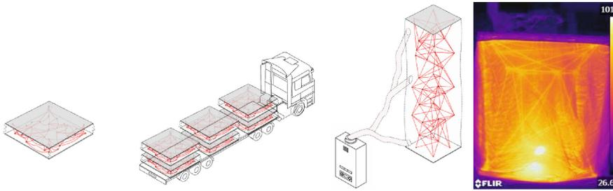
**Fig. 16.** **a** Transportation and deployment strategy of a wound structure **b** Thermal image of prototype in deployable oven
