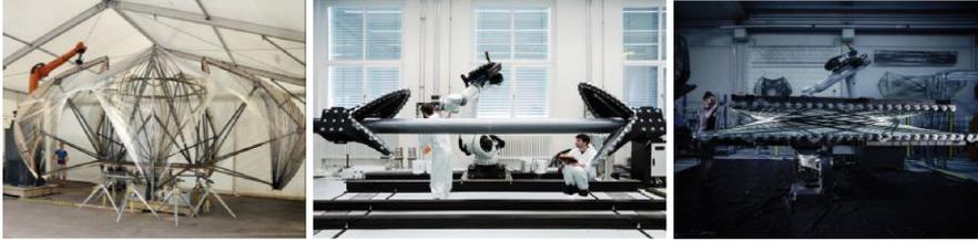
**Fig. 1.** Winding frames of: **a** ICD/ITKE Research Pavilion 2012 (Knippers et al. 2015) **b** BUGA Fiber Pavilion (Menges et al. 2022) **c** Maison Fibre (ICD and ITKE 2021)
