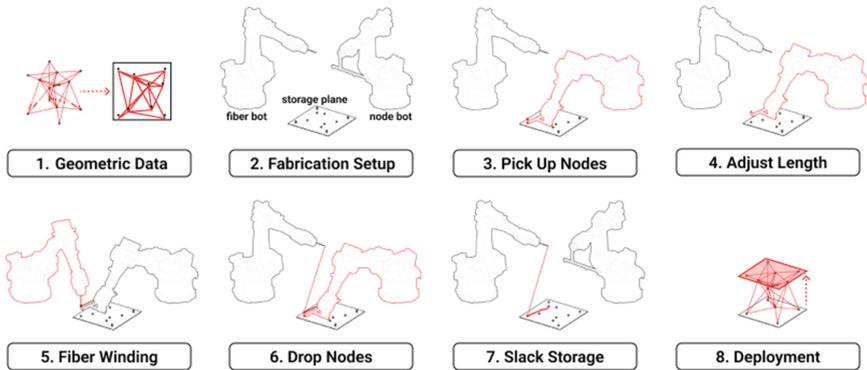
Fig. 7. Fabrication sequence of *Slack Pack* system
