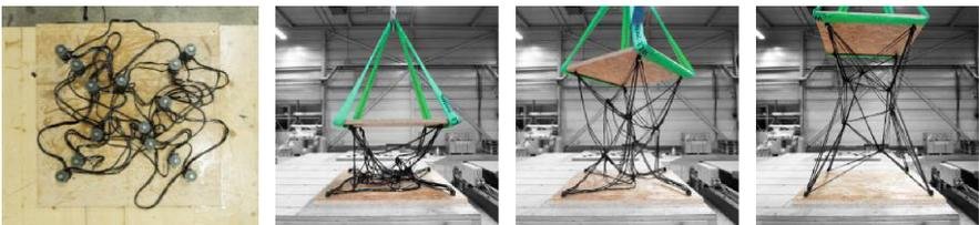
**Fig. 20.** **a** Aerial view of fabrication setup **b** Robot winding sequence including picking up nodes, winding fiber member, and returning nodes and wound member to storage plane.
