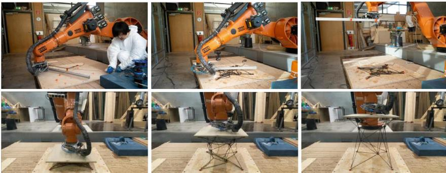
**Fig. 17.** **a** Semi-robotic winding of early prototype **b** Deployment of prototype structure
