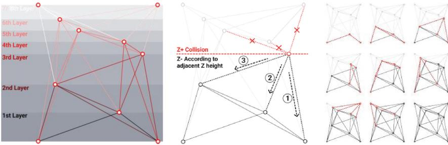
Fig. 8. a Winding layers b Winding order within winding layer c Overall winding order
