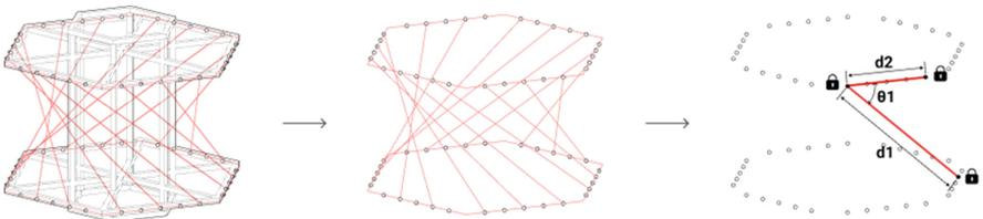
**Fig. 4.** **a** Conventional winding frame in CFW **b** Location of anchor points **c** Geometric relationships of anchor points
