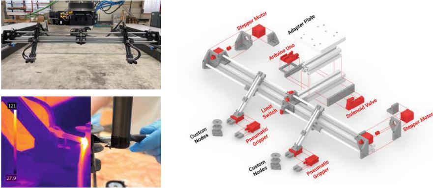
**Fig. 15.** a End effector installed on the robot b Resistive curing and thermal imaging of node c Exploded view of end effector
