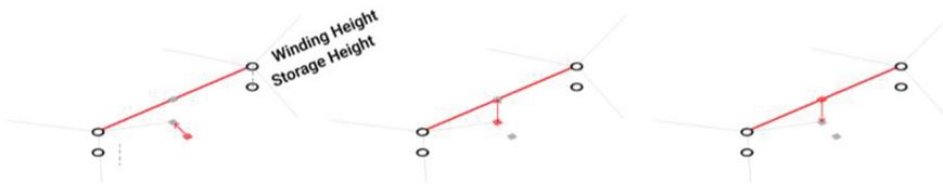
**Fig. 14.** Toolpath generation for NodeBot **a** Node pickup position at correct offset **b** Raise nodes to winding height **c** Return nodes to storage plane
