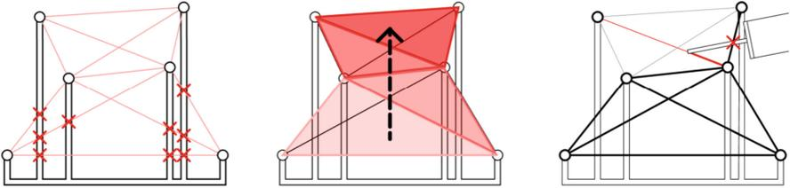
**Fig. 3.** **a** Fiber colliding with frame **b** Robot reachability decreasing (red areas) with the addition of members **c** Robot colliding with upward pointing members
