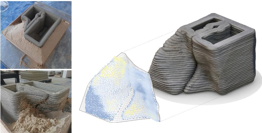
**Fig. 7.** Section print test of one of the prototypes, using sand as support material (left) and analysis of the photogrammetry model obtained with the target geometry (right).
