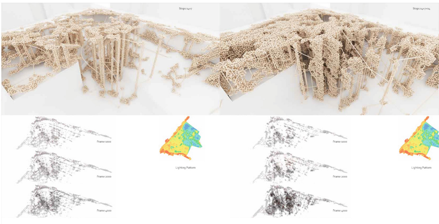
Fig. 6. Discrete set of 3D points (Processing) from solar radiation patterns (using Ladybug) being translated by a weaving process (Grasshopper), in a linear process (left) and in a recursive process (right) showing different densities and complexities. Image from the Authors.
