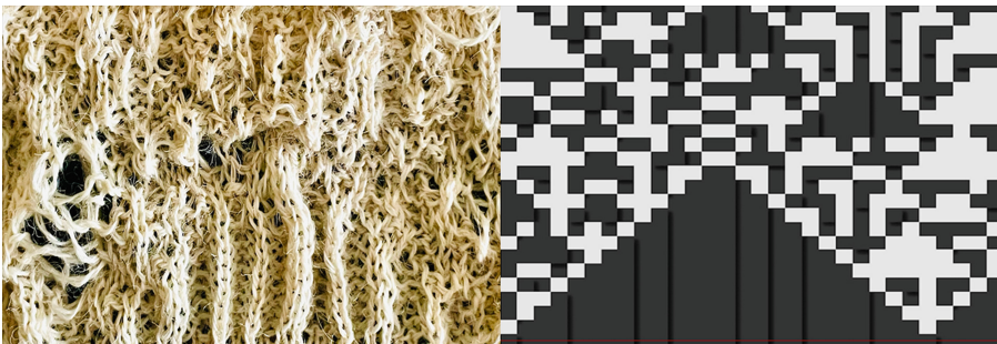
Fig. 7. 3D Knitted CA sample (Ecological Wool 2/14 Nm) based on the 30 \times 30 from a 2.5D CA system (CA 2.5D Game of Life) being made using a Digital Knitting Machine (Kniterate). Image from the authors.
