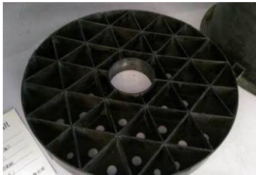
Fig. 7 Mirror body with carbon fiber grid reinforced structure.
