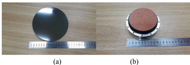
Fig. 9 Workpiece and polishing tool for experiments: (a) 150-mm RB-SiC and (b) 100-mm RC lap.
