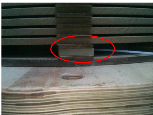
Fig. 5 FBG-based pressure sensor installation diagram.
