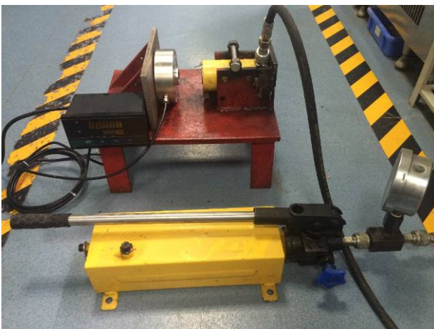
Fig. 3 Pressure sensor test system flow chart and picture.
