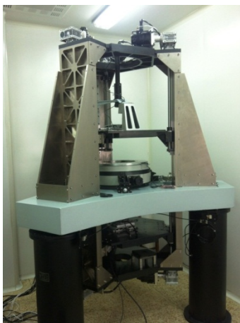
Fig. 8 Experimental lateral shearing interferometer.
